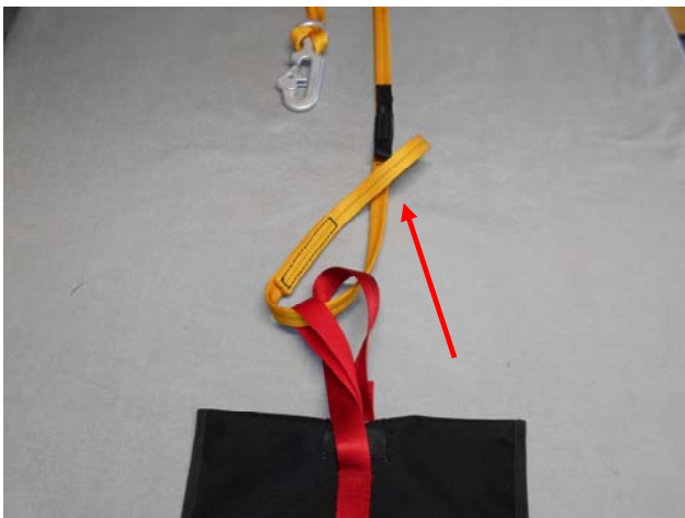
Pass the Hook of the Static Line through the loop of the tail end of the Static Line .
