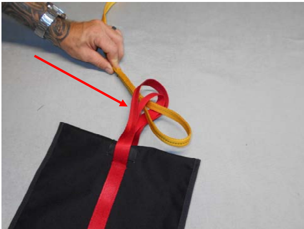
Pass the tail end of the Static Line (TPDS-G12-211) through the two loops of the Static Line Pouch.
