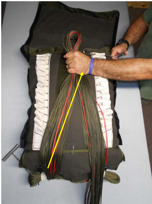
Pull the Suspension Lines from the top of the D-bag across towards the opposite far end.
