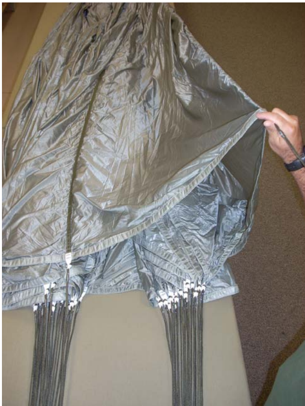
Flake one side of the canopy. Be sure to clear the material from between the lines.
