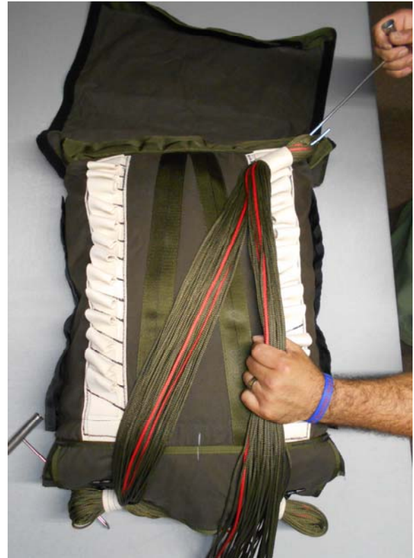
Stow a bight of the line in the first Cotton Loop.
