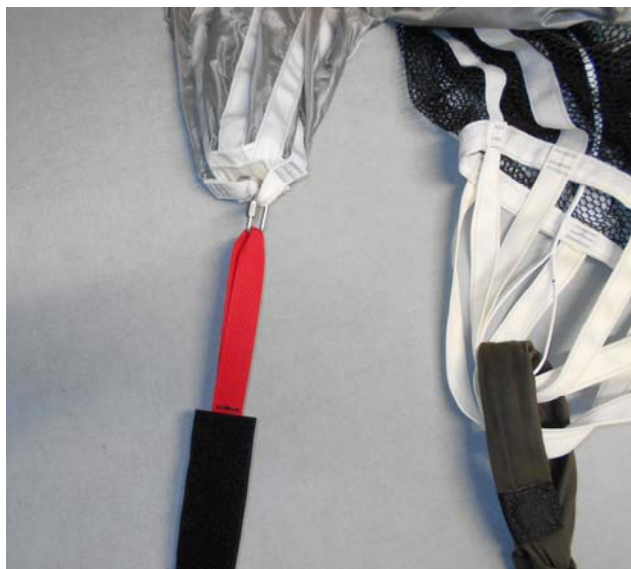
Pictured above is the S/L Pile Velcro Connector (A) (TPDS-G12-210) attached to the Drogue.
