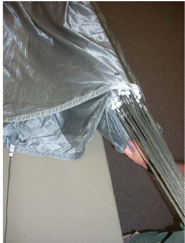
Continue until all panels of that side of the canopy are flaked.
