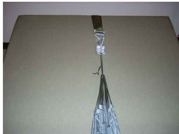
Hook up the apex to the table ring or hook. Square the Apex.
