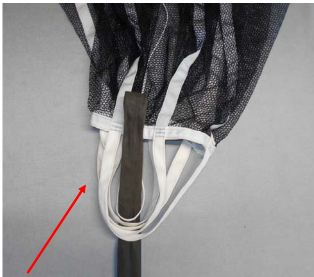
Pass the tail of the Drogue Bridle through the loops of the Drogue and the loop of the Center Line.
