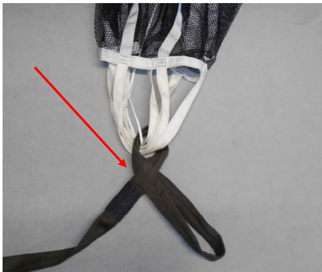
Pass the end of the Bridle through the small loop of the bridle.
