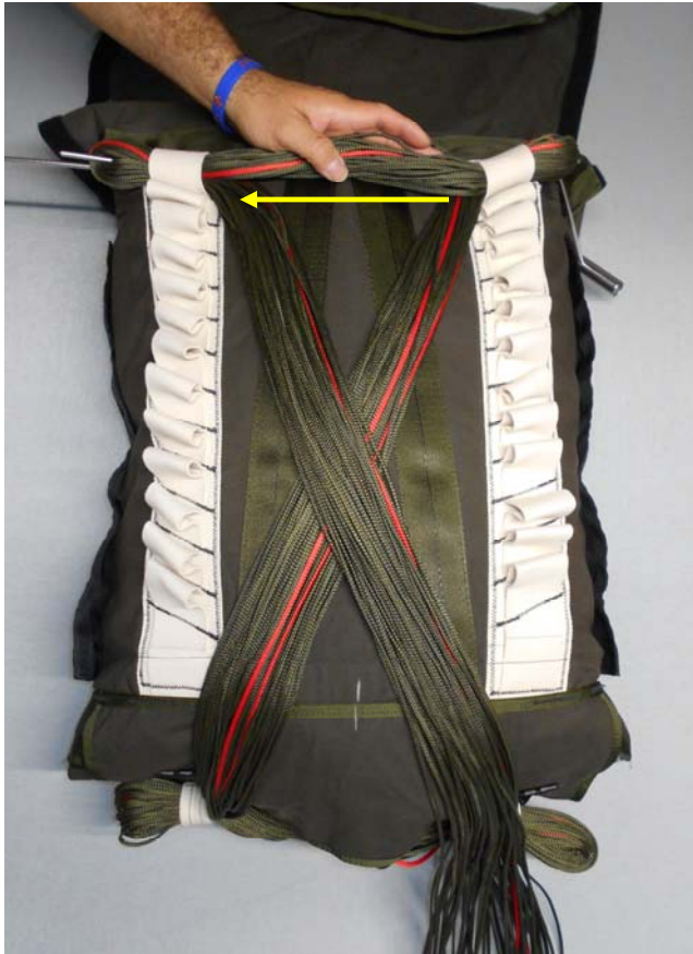
Stow another bight of the line in the Cotton Loop across from the first.
