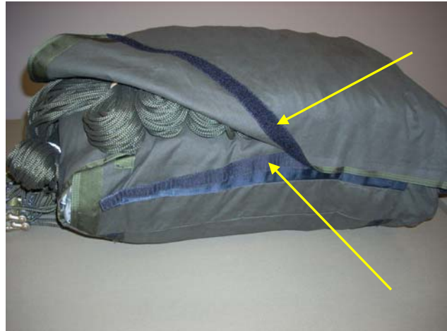
Mate the hook and pile Velcro on the sides of the Deployment Bag.
