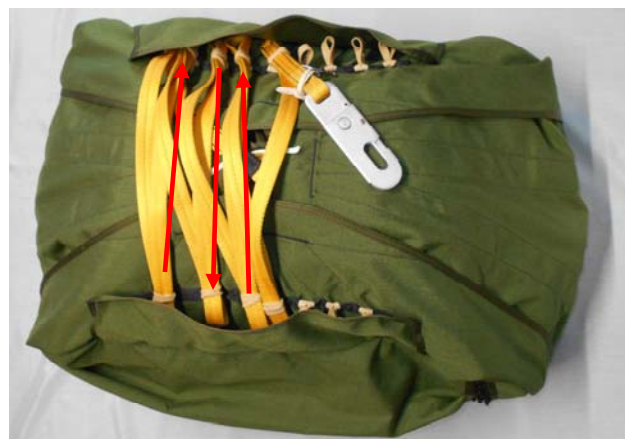
Continue to stow the Static-Line back and forth with about 2" in each rubber band.
