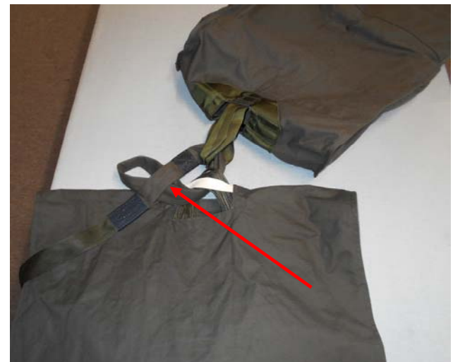
Pass the end of the bridle through the small loop of the bridle.
