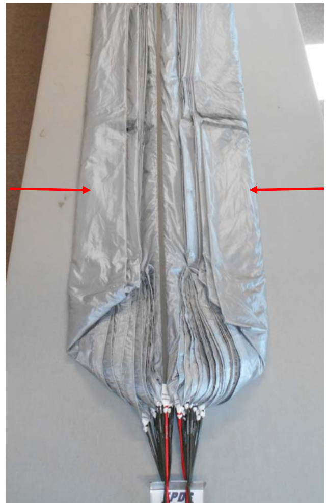
Fold the flaked gores to the center of the parachute.
