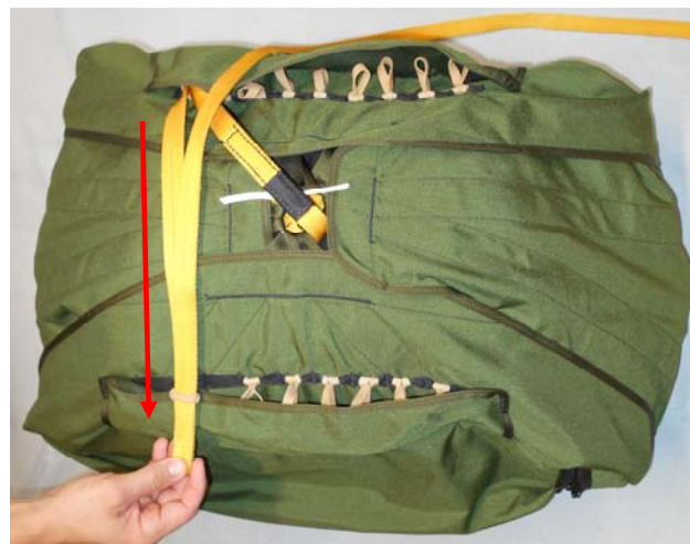
Stow 2" of a second bight of the Static-Line in a rubber band opposite of the first.
