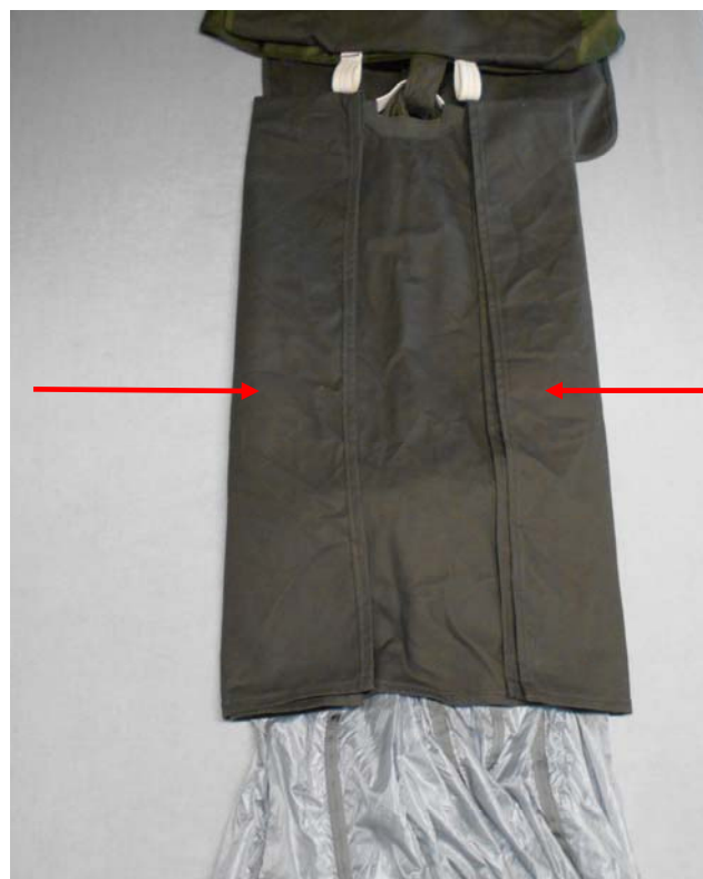
Fold the sides to the center.
