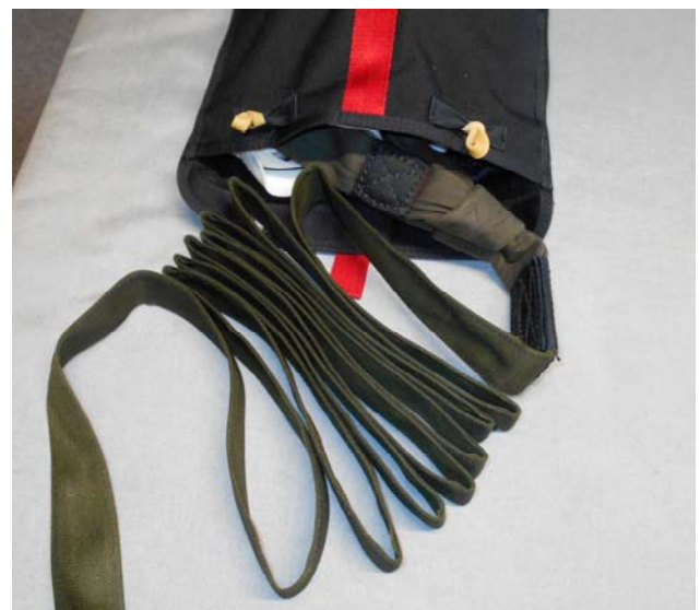
“S”-fold the Drogue Bridle as shown.
