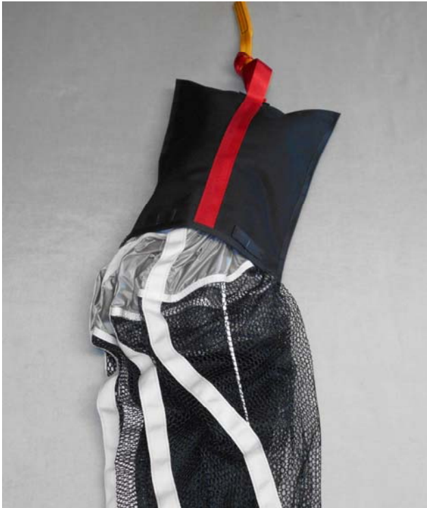
“S”-fold the Drogue into the Pouch.
