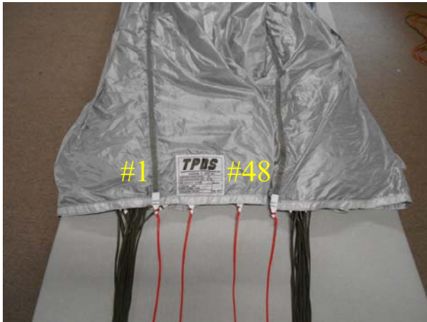
Pictured above is the top of the Cargo Parachute. Red lines indicate lines #1, #24, # 25, & #48.
