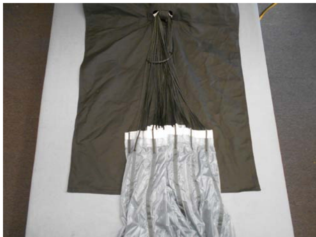
Straighten and square the Apex Cover to the Parachute and Apex lines.
