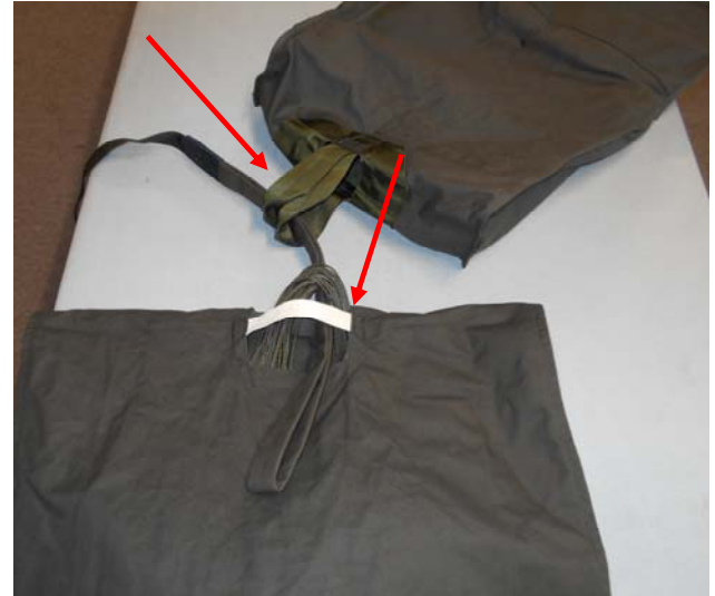
With the D-bag turned inside-out pass the Drogue Bridle through the T-8 loops then through the apex lines, then under the apex cover loop.
