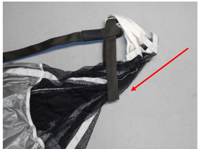
Pass the Drogue through the opened loop of the Drogue Bridle.
