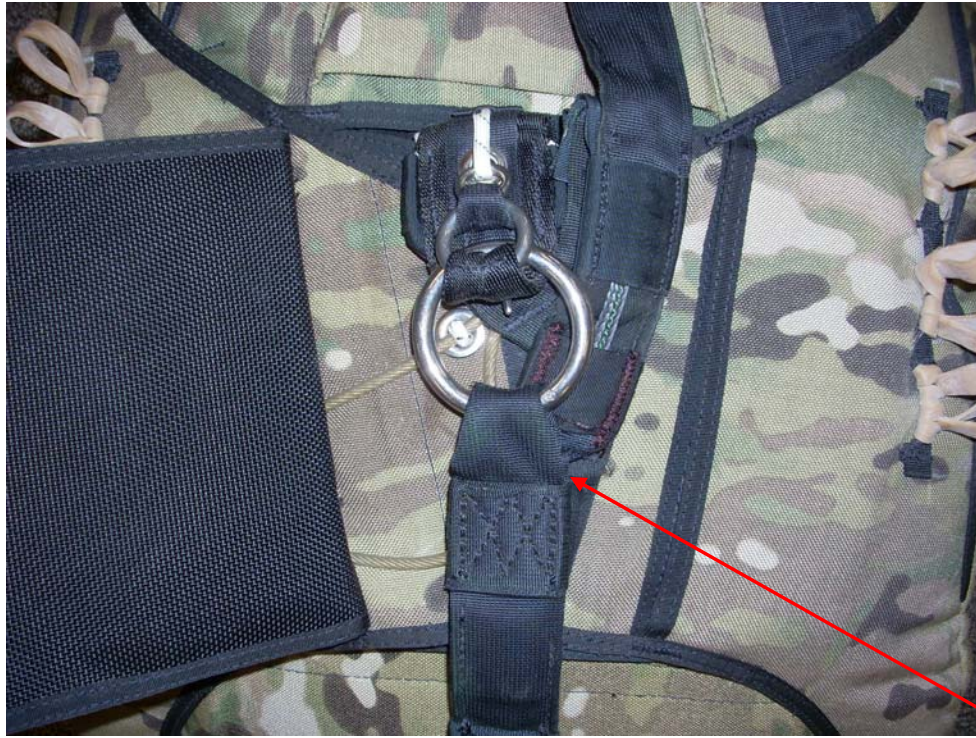
TPDS Heavy Load Tactical (HLT) with Replaceable 3-Ring Drogue Riser.
